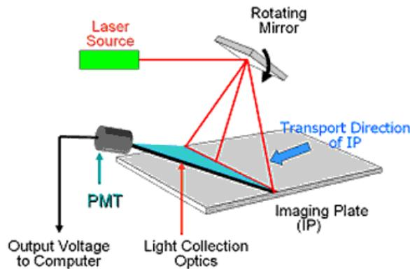
Fig 6: Schematic of the steps involved with CR imaging.
