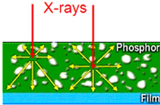
Fig 1: X-rays (red) absorbed by phosphor and converted to visible light (yellow).
