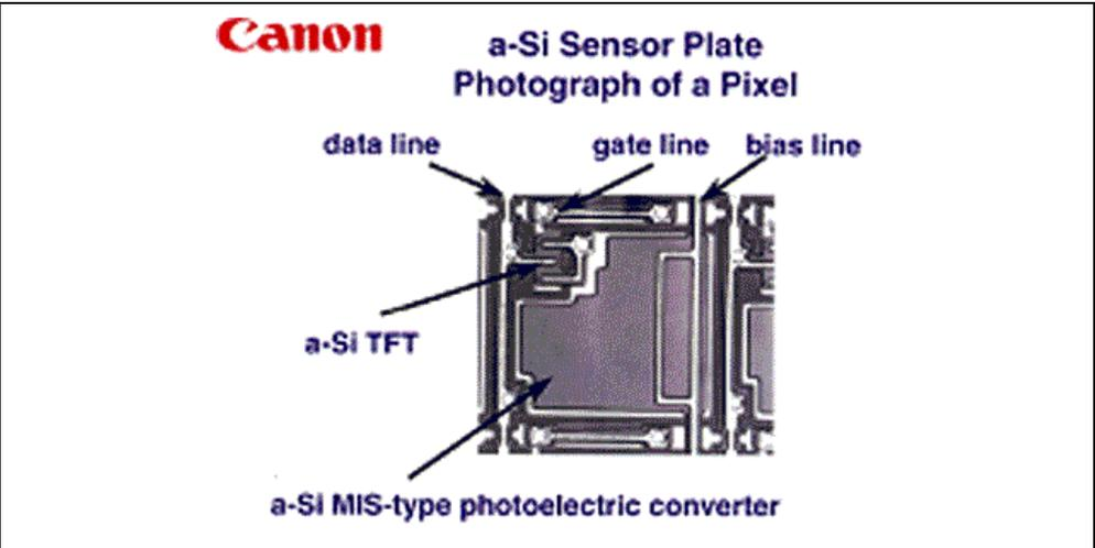
Fig 10: Photograph of individual a-Si pixel. Courtesy Cannon Medical Systems
