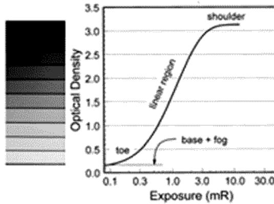
Fig 3: Gray level (O.D.) of film vs. x-ray exposure (mR). Note semi-logarithmic graph.
