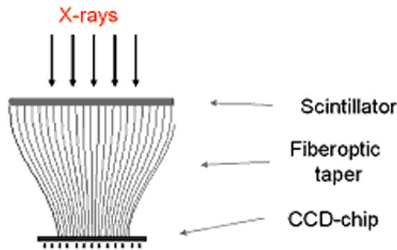
Fig 7: Schematic of a charge-coupling device acquiring an x-ray image.
