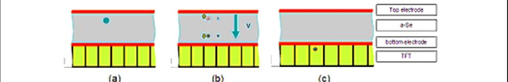
Fig 11: Direct capture detector: (a) Capture of x-ray by a-Se; (b) conversion of x-ray into electron-hole with applied voltage  $V$ ; (c) detection of charge by TFT
