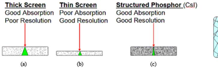
Fig 2: (a) Thicker phosphor absorbs more x-rays but has reduced resolution as compared to (b). (c) Cesium iodide (CsI) phosphor are long crystalline needles, maintaining resolution with good absorption efficiency (far right single CsI crystal with light propagation shown).
