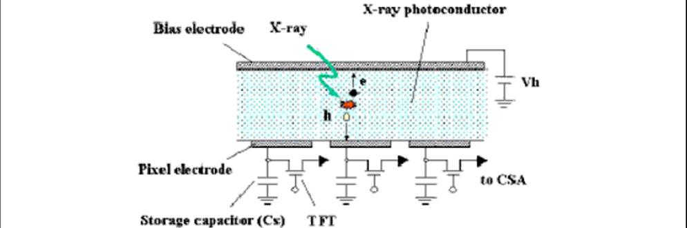
Fig 12: Diagram of electronic components of a direct capture detector with 3 pixels shown.  $V_h$  is the applied voltage and CSA refers to computer system analysis.
