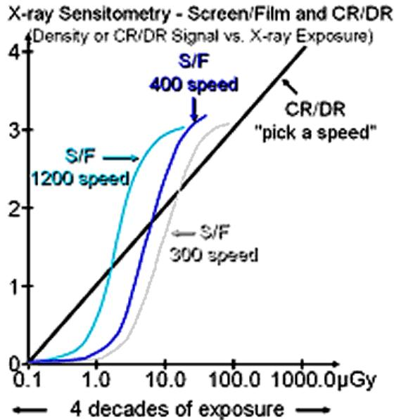
Fig 4: H&D curves for different screen-film speed systems and for digital detectors.
