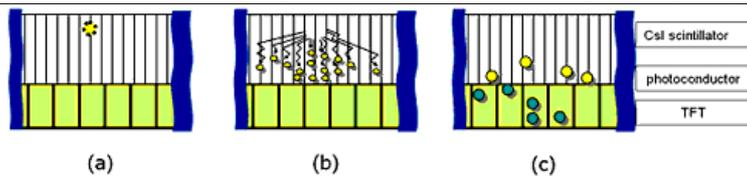
Fig 8: Illustration of indirect digital imaging: (a) x-ray interacting with CsI phosphor; (b) conversion of x-ray to visible light by scintillator (exaggerated light spread for clarity); (c) conversion of visible light to electrons and capture of electrons by TFT
